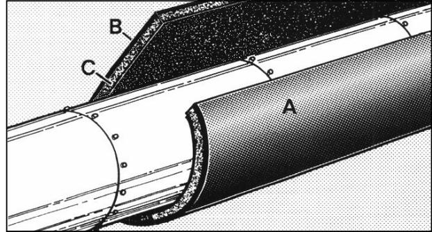
***BM-1C IS USED AS AN EXTERNAL 'WRAP' OR LIMP MASS BARRIER WITHIN STRUCTURES TO CONTROL NOISE LEAKAGE OR PENETRATION.***
